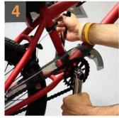
To check your bottom bracket/ crank; grab each crank arm and wiggle from side to side. If there is any play in the arms or the bottom bracket, don't ride and head into the shop!
