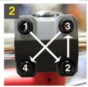
Using the proper sized metric allen key, check to see if your stem bolts are tight. If you need to tighten them do so using the pattern above.
