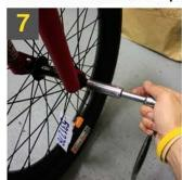
Using proper sized socket or wrench, make sure your axle nuts are tight. If you have pegs you will need a socket extention.
