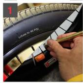
Recommended tire pressure is shown on the side of the tire. Inflate your tires to the proper pressure before each ride!
