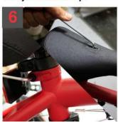
Make sure your seat/ seat collar is tight. Using The proper sized allen key tighten your seat collar if needed. If you have a pivitol seat use the slit in the top of the seat to tighten the seat to the post.
